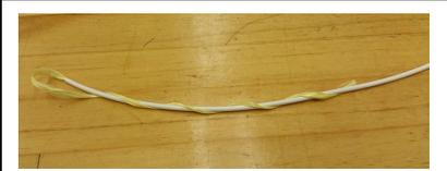
**Step 3.** Secure the aramid to the cordage with vinyl tape. The cable is now ready for installation.
